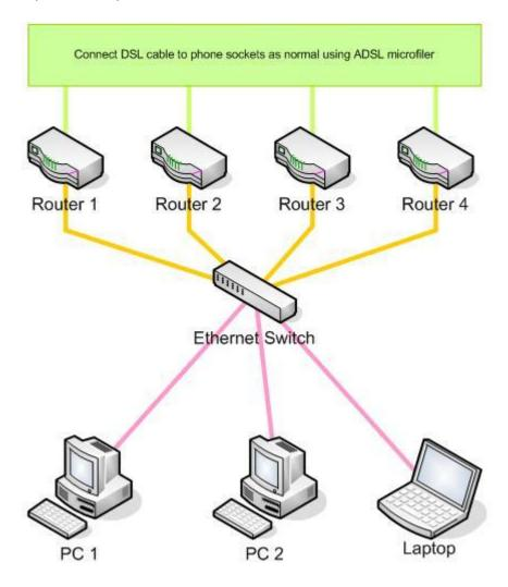
Routers 1 - 4 are able to communicate with each other via the switch. This allows the bonded DSL software to make use of all routers and route traffic according to the performance of each line.
