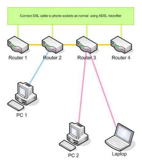
While everything is working, this will still give you all the benefits of the bonded setup with the aggregated bandwidth of all lines and the service will continue to operate with the remaining lines, if there is a failure on any line.
